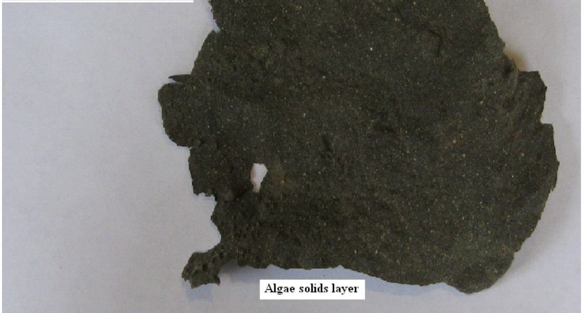
Chemically dewatered solids
